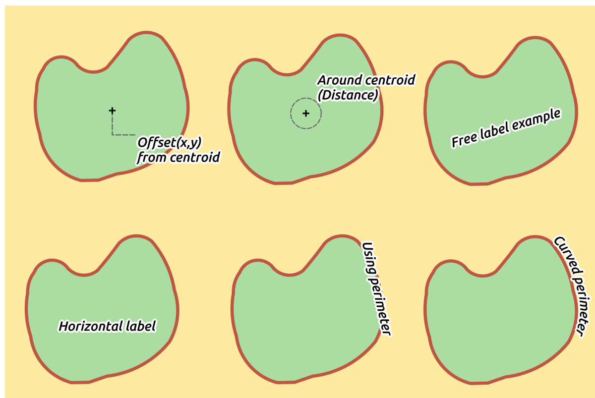
Figure 12.32: Label placement examples in polygons
